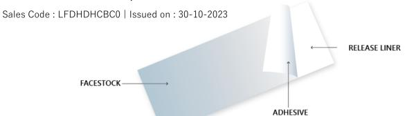
FACESTOCK BOPP (Biaxially Oriented Polypropylene) Metalize Silver Film
